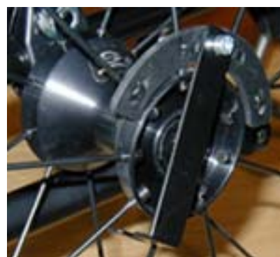
Figure 2. Unlocked position – now the wheel cannot be removed.
