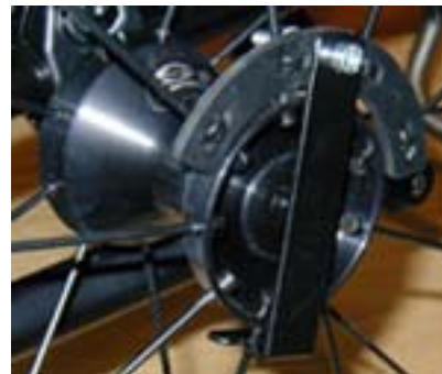
Figure 1. Locked position –the wheel can now be removed. The locking plate is attached around a spoke.
